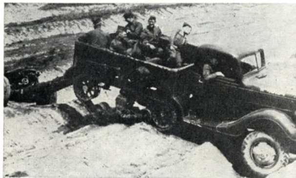
Half-Track Truck T9E1 was standardised as the M2 and built by Marmon-Herrington. It is here seen as an artillery tractor in 1939.
